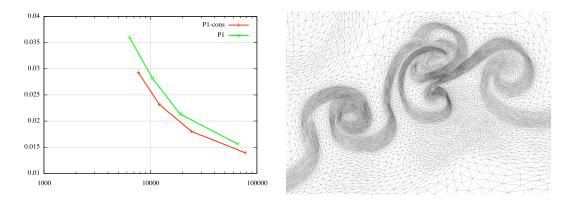
Figure 20. Left,  $\mathbf{L}^2$ -norm error of the density with respect to the reference solution for adaptive simulations for  $\varepsilon$  from 0.05 to 0.02. In red, adaptive simulations with the  $\mathbf{P}^1$ -conservative interpolation and, in green, with the  $\mathbf{P}^1$  interpolation. Right, a close up view of the adapted mesh of Figure 18 (top) in a region where instabilities occur.
