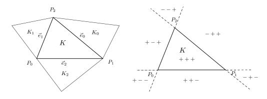
Figure 1. Left, definition of a triangle K and its three neighbors  $K_i$ . Vertices indices are ordered counter-clockwise and the entities numeration is the same as the viewing vertices. Right, the seven regions defined by the signs of the three barycentric coordinates of a point P with respect to an element K.
