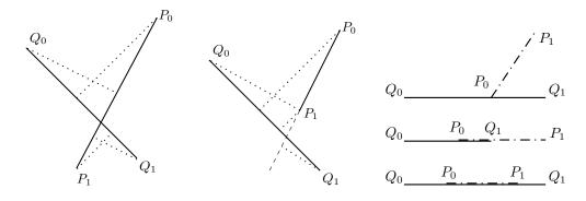
Figure 8. Edge-edge intersection cases: an intersection (left), no intersection (middle) and several degenerated cases (right).
