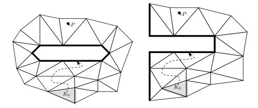
Figure 4. Starting element  $K_0$  and vertex P are separated by a hole (left) or the non-convex domain (right). The path demands to pass through the hole or the boundary to reach the element containing vertex P.
