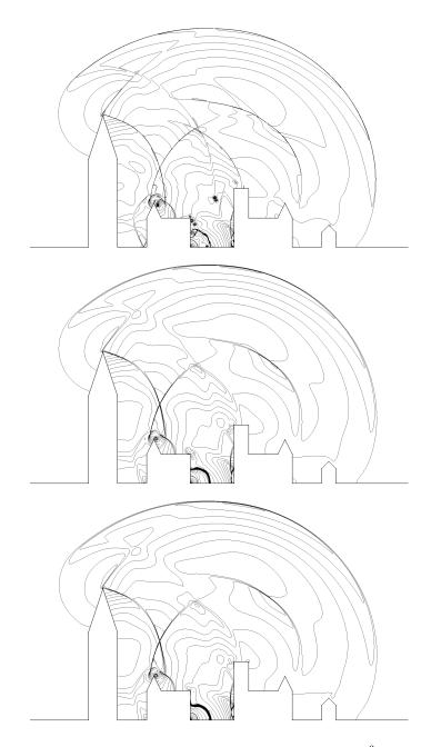
Figure 24. Density isolines from 0.085 to 0.19 with an increment of  $2.65 e^{-3}$  at time t = 0.2 seconds. Top, the reference solution, i.e.,  $\varepsilon = 0.003$  and the  $\mathbf{P}^1$ -conservative interpolation. Middle, adapted solution obtained for  $\varepsilon = 0.006$  with the  $\mathbf{P}^1$ -conservative interpolation. Bottom, adapted solution obtained for  $\varepsilon = 0.006$  with the  $\mathbf{P}^1$ -interpolation.
