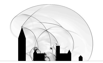
Figure 21. A schlieren type picture representing the final density at t = 0.2 sec on the final adapted mesh containing 170,020 vertices obtained from an error level of 0.003 and the  $\mathbf{P}^1$ -conservative interpolation.
