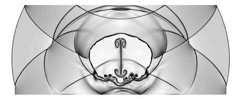
Figure 17. A schlieren type picture representing the final density at t = 0.7 on the final adapted mesh containing 158, 121 vertices obtained from an error level of 0.015 and the  $\mathbf{P}^1$ -conservative interpolation.
