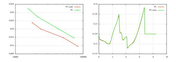
Figure 25. Left,  $\mathbf{L}^2$ -norm error of the density with respect to the reference solution for adaptive simulations for  $\varepsilon$  from 0.007 to 0.004. In red, adaptive simulations with the  $\mathbf{P}^1$ -conservative interpolation and, in green, with the  $\mathbf{P}^1$  interpolation. Right, comparison of the density profile at time t = 0.2 seconds along the line of equation y = 3.07692x - 17.4615 for the solutions obtained with an error threshold  $\varepsilon = 0.006$ .
