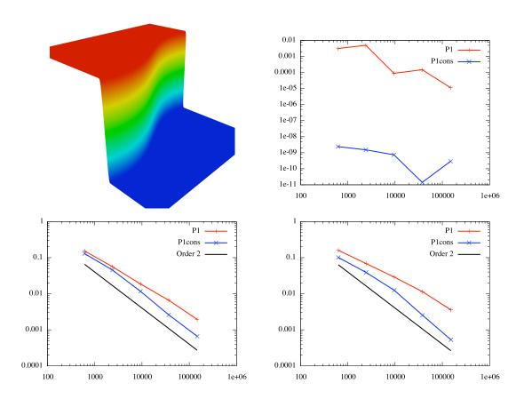
Figure 13. Continuous sinusoidal shock analytical function  $f_2$ . Top left, a three-dimensionnal representation of the function. Top right, the mass variation for the transfer  $\mathcal{H}_i^1 \to \mathcal{H}_i^2$ . Bottom left, the error  $\varepsilon_i$  for the transfer  $\mathcal{H}_i^1 \to \mathcal{H}_i^2$ . Bottom right, the error  $\epsilon_i$  for the transfer  $\mathcal{H}_i^1 \to \mathcal{H}_i^2 \to \mathcal{H}_i^1$ .
