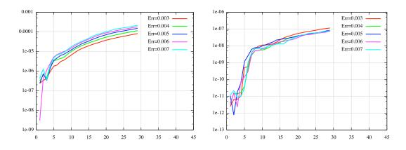
Figure 26. Density relative mass variation during the simulation for all cases. The abscissae represent the iterations of the mesh adaptation algorithm. Left, mass variation for the  $\mathbf{P}^1$  interpolation. Right, mass variation for the  $\mathbf{P}^1$ -conservative interpolation.
