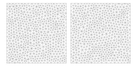
Figure 11. Uniform unstructured triangular meshes used to compare interpolation schemes. Left,  $\mathcal{H}_1^1$  containing 631 vertices, and right,  $\mathcal{H}_1^2$  containing 611 vertices.
