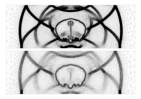
Figure 18. Final adapted meshes using the  $\mathbf{P}^1$ -conservative interpolation at time t = 0.7 for errors equal to 0.015 (top) and 0.03 (bottom). The upper mesh contains 158, 121 vertices and the lower one 24, 297.
