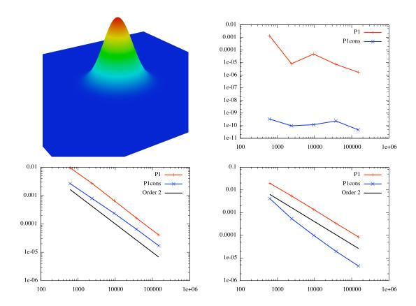
Figure 12. Gaussian analytical function  $f_1$ . Top left, a three-dimensionnal representation of the function. Top right, the mass variation for the transfer  $\mathcal{H}_i^1 \to \mathcal{H}_i^2$ . Bottom left, the error  $\varepsilon_i$  for the transfer  $\mathcal{H}_i^1 \to \mathcal{H}_i^2 \to \mathcal{H}_i^1$ .
