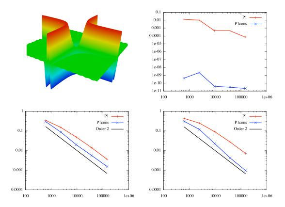
Figure 14. Multi-scales smooth analytical function  $f_3$ . Top left, a three-dimensionnal representation of the function. Top right, the mass variation for the transfer  $\mathcal{H}_i^1 \to \mathcal{H}_i^2$ . Bottom left, the error  $\varepsilon_i$  for the transfer  $\mathcal{H}_i^1 \to \mathcal{H}_i^2$ . Bottom right, the error  $\epsilon_i$  for the transfer  $\mathcal{H}_i^1 \to \mathcal{H}_i^2 \to \mathcal{H}_i^1$ .
