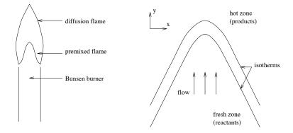
FIG. 1. Bunsen flames (left) and the premixed flame (right).
